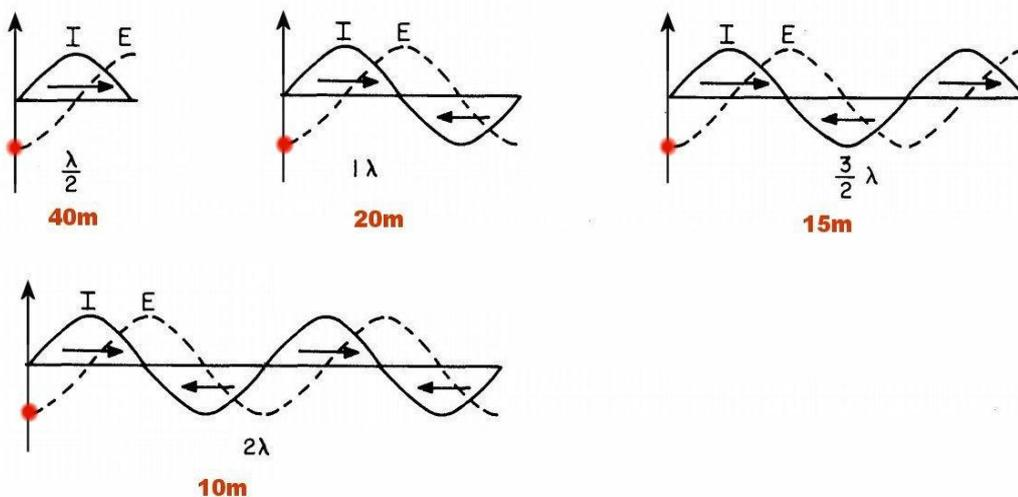
Plot of voltage (E) and current (I) in a conductor 20 meters long
