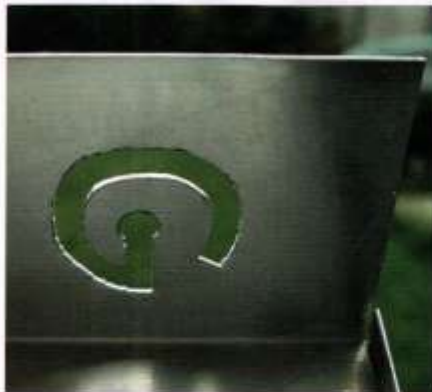
PHOTO 2: Cutting the round hole for the meter movement.
