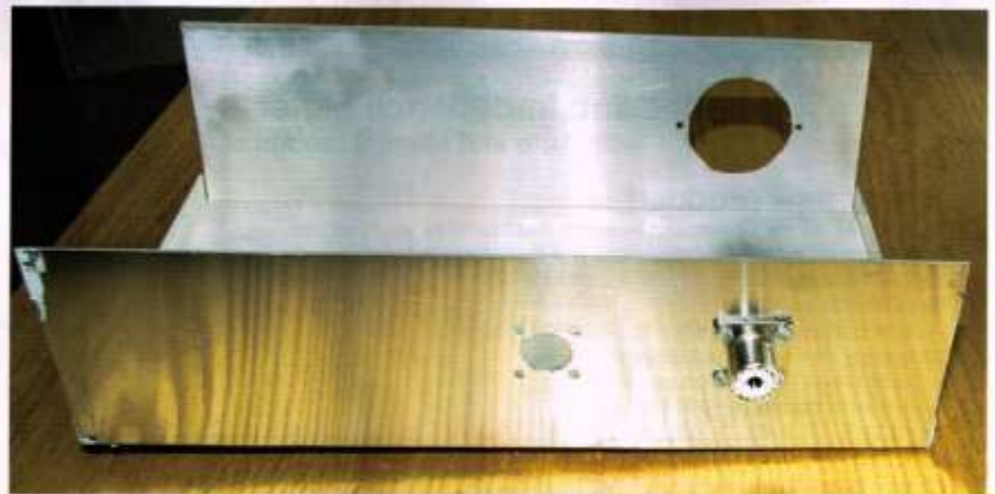
PHOTO 3: Rear panel, with one socket installed.
