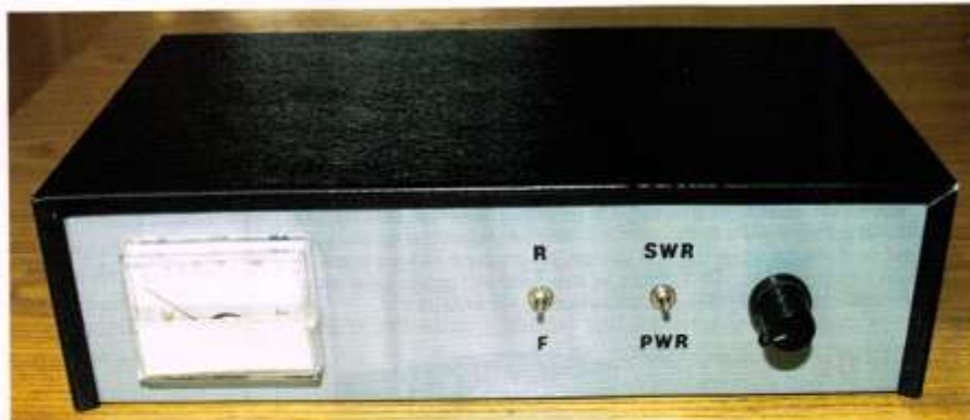
PHOTO 4: The finished power/SWR meter.
