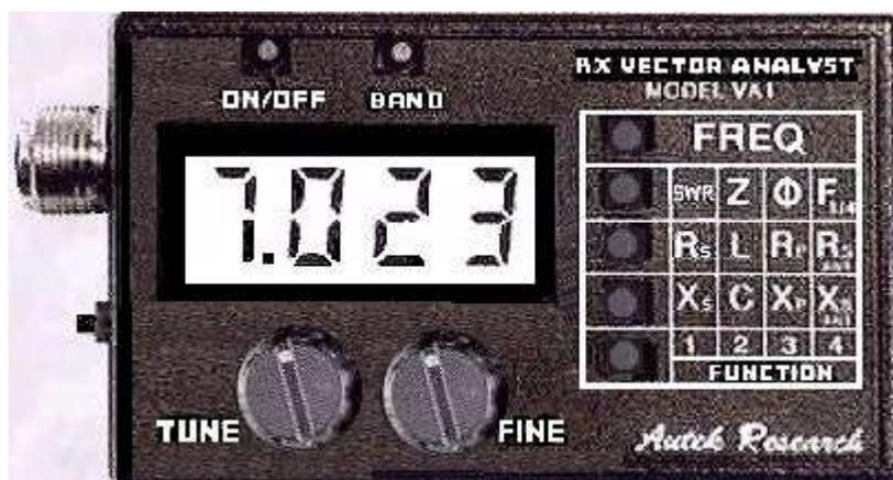
The pocket-sized VA1 is designed to check and adjust antennas, feedlines, and RF networks. It includes a microprocessor, A/D converters, and a low-power "transmitter" with 4 digit frequency readout, continuously variable from 0.5 to 32 MHz in 6 bands. Like its little brother, the RF1, it measures RF values of true impedance (0-1000 ohms), SWR (1 to 15:1), C (0-
