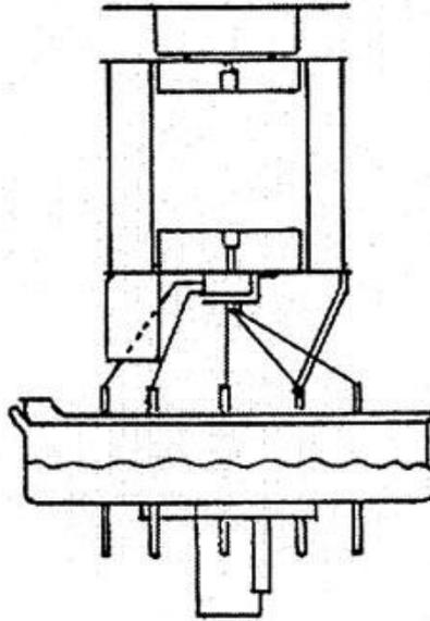
**Figure 3: Construction of EF50.**
