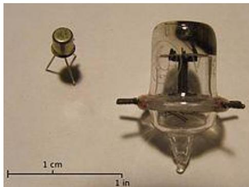
An acorn valve alongside a bipolar transistor
