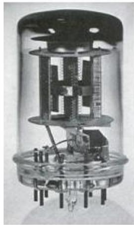
**Original EF50 sample as supplied to PYE electronics**
