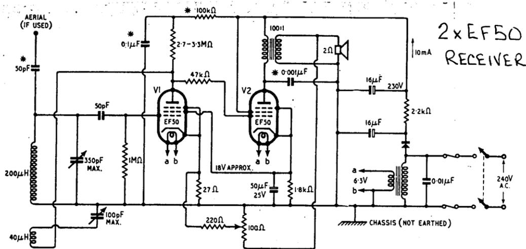
Circuit diagram of the receiver. Resistors can be  $\frac{1}{2}$ W and capacitors 350V d.c. working. The 0.01- $\mu$ F capacitor across the mains input must be capable of continuous operation at 250V a.c. Components marked thus \* may be omitted for "local" reception. The cathode resistor for V<sub>2</sub> must be adjusted to fix the h.t. current at 10 mA.
