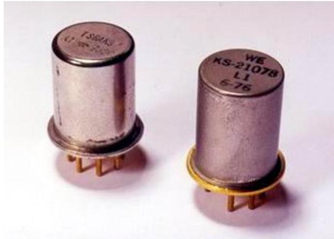
These were JFET based devices made into little metal cans with pins poking out the bottom. They were replacements for tubes (Valves to us DownUnder) and as far as I can find out Fetrons were made to replace at least the following common valve types. 6AK5 or 408A, 6AM6, 6CB6A, 12AT7, 12AU7 and 12AX7. There were also many more that replaced the specialised tubes in telephone exchange equipment.
